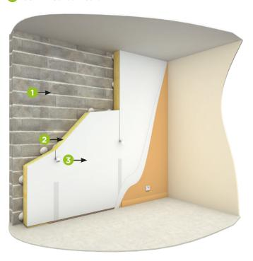
\*Adhesive dabs should be applied in a regular pattern in accordance with EN 8212: 1995 and EN 8000 Part 8: 1994 to give a minimum area of contact between board and background of 20%.
